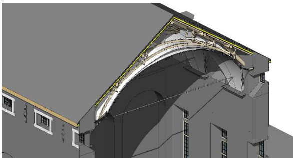
Figure 7 The Oratorio degli Uomini , one of the main wings to be renovated, BIM model (R. Babbetto). The design solution previews a new insulating layer under the roof.
