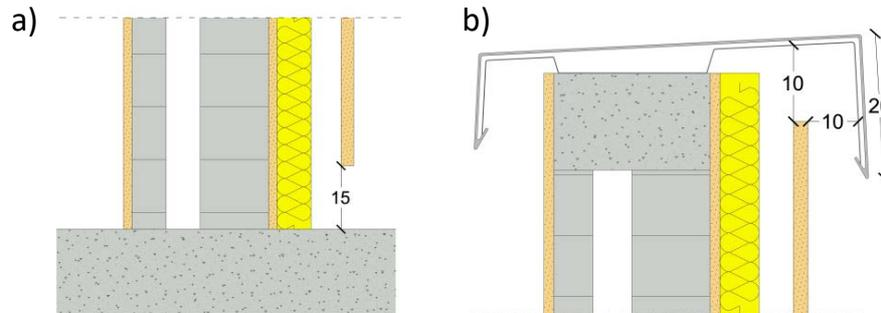
**Figure 6.** Inlet (a) and outlet (b) sections of ventilated facade. All measures are expressed in cm
