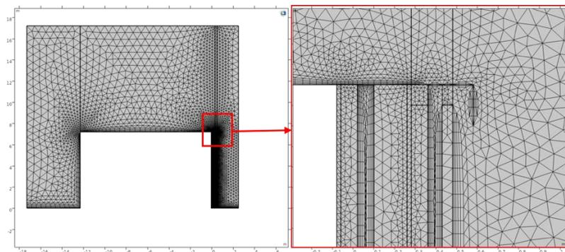
**Figure 7.** Physics-controlled mesh with free triangular geometry.
