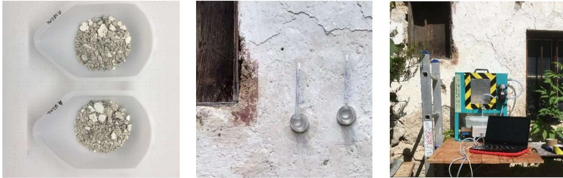
Figure 3. From left to right, samples for gravimetric analysis, Karsten tubes and WAM100-B
