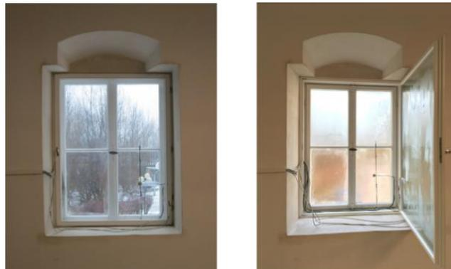
Figure 2. Interior view of window F 1.27 with closed (left) and open inner window casement. A heat flow sensor can be seen in the middle of the lower right glazing.
