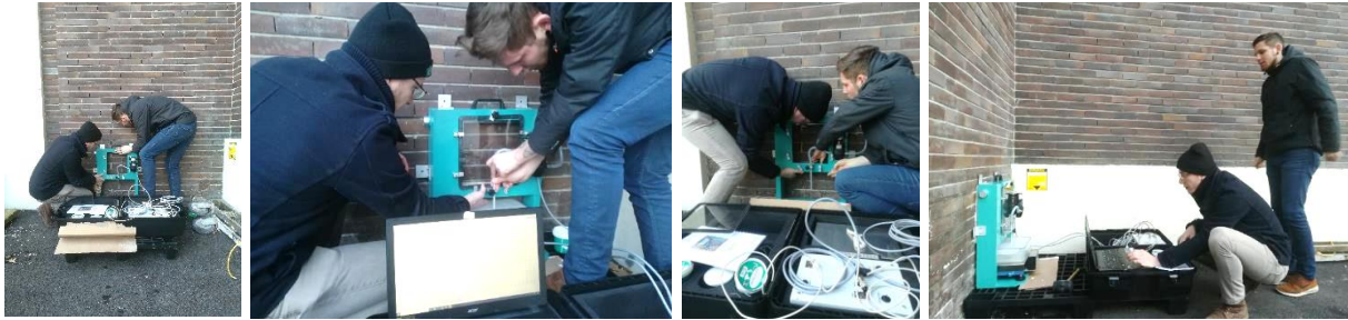
Figure 5. Measuring the water uptake of a façade in-situ during the application week in the hygrothermal testing lab at EURAC Research in Bozen/Italy. (Photo: A. Troi 2019)
