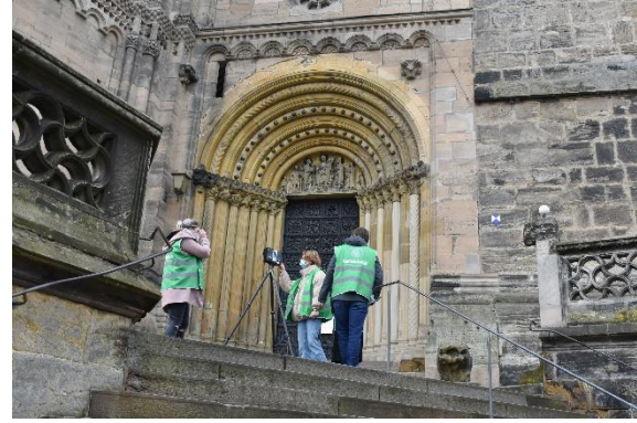
Figure 4. A 3D terrestrial laser scan and spherical targets are prepared by students at one of the main portals of Bamberg Cathedral. (Photo: M. Hess 2021)
