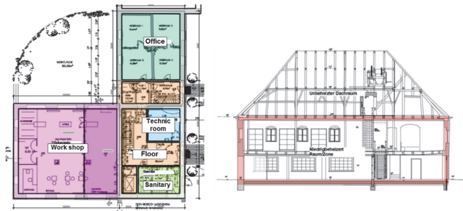
Figure 3. Multi zonal model of the ground floor (left) and cross section of the Alte Schöfflerei (right) with boundary of heated space (red line).
