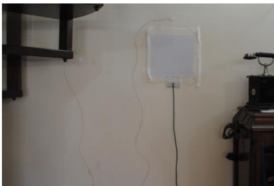
Figure 3. Heat flow meter in mp1.
